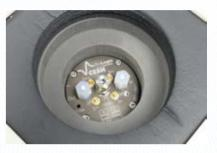
The sample can be prepared in a glove box, placed in the **CESH** and then installed in the **ITS**. The **ITS** is compatible with **MTZ-35 impedance analyzer** and with Bio**Logic** potentiostats/galvanostats/FRAs. This allows Bio**Logic**
